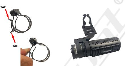
1 - To install the dashcam into the mount, simply squeeze the two tabs of the spring clip together as shown above. This will increase the diameter of the spring clip and allow you to slide the dashcam into position. Once the dashcam is in position, release the two tabs. The dashcam is now securely attached to the mount.
