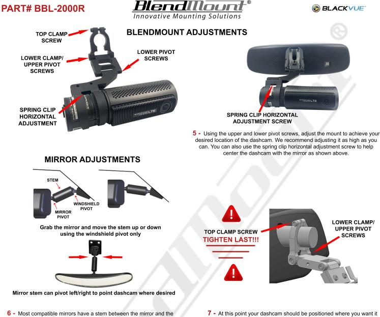
Most compatible mirrors have a stem between the mirror and the windshield that has a pivot on both ends. To adjust the mirror up or down, grab the mirror and move the stem up or down using the windshield pivot only. Adjust the mirror to your normal viewing position using the mirror pivot only. Notice the different location of the mirror shown above.
